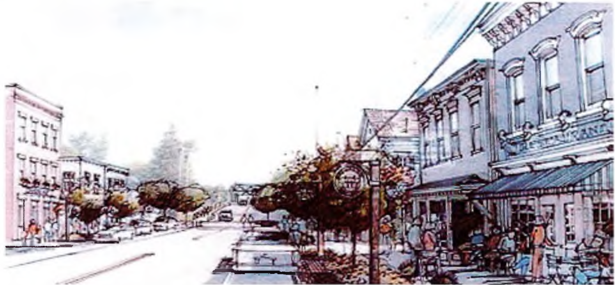
Proposed downtown Main Street. Note the improved façade treatments, sidewalks, banner poles, street trees, and signage. Note also the slight narrowing of Route 11 to enlarge the sidewalks, organize the parallel parking, and calm through traffic.
